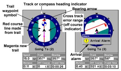
Navigate trail, navigation page (compass rose) views: driver (left) is heading north straight toward trail point 2; bearing arrow shows the trail point is 357 degrees (straight ahead.) Driver (right) has reached trail point 2 and must turn northeast to follow the trail. Arrival alarm goes off and bearing arrow swings around to say turn right (east), toward the next waypoint, trail point 3. The unit now shows navigation information to point 3, which is 0.40 miles away.
